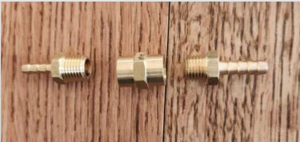
Figure 1. Coupling Assembly for joining two plastic tubings
