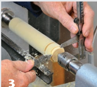
3 Part the tenon shoulders down to a slightly oversized diameter.
