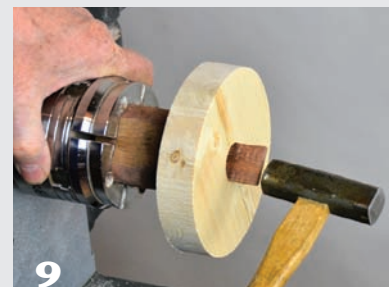
An undersized tenon on the jam chuck can be tightened with a wedge driven into a saw kerf.
