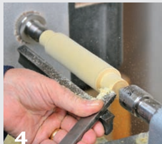
4 Trim the tenon with a skew chisel. Practice and patience combine for a perfect fit.
