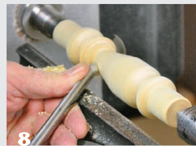
Working from the tailstock toward the headstock, shape the spindle elements with a gouge and skew chisel.
