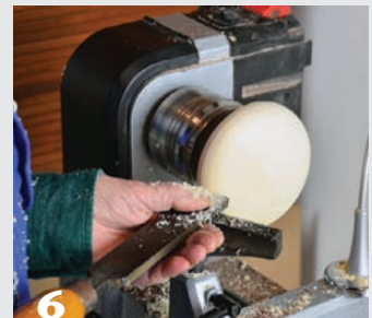
6 A freshly sharpened scraper produces paper-thin shavings and a smooth surface on the face-turned discs.
